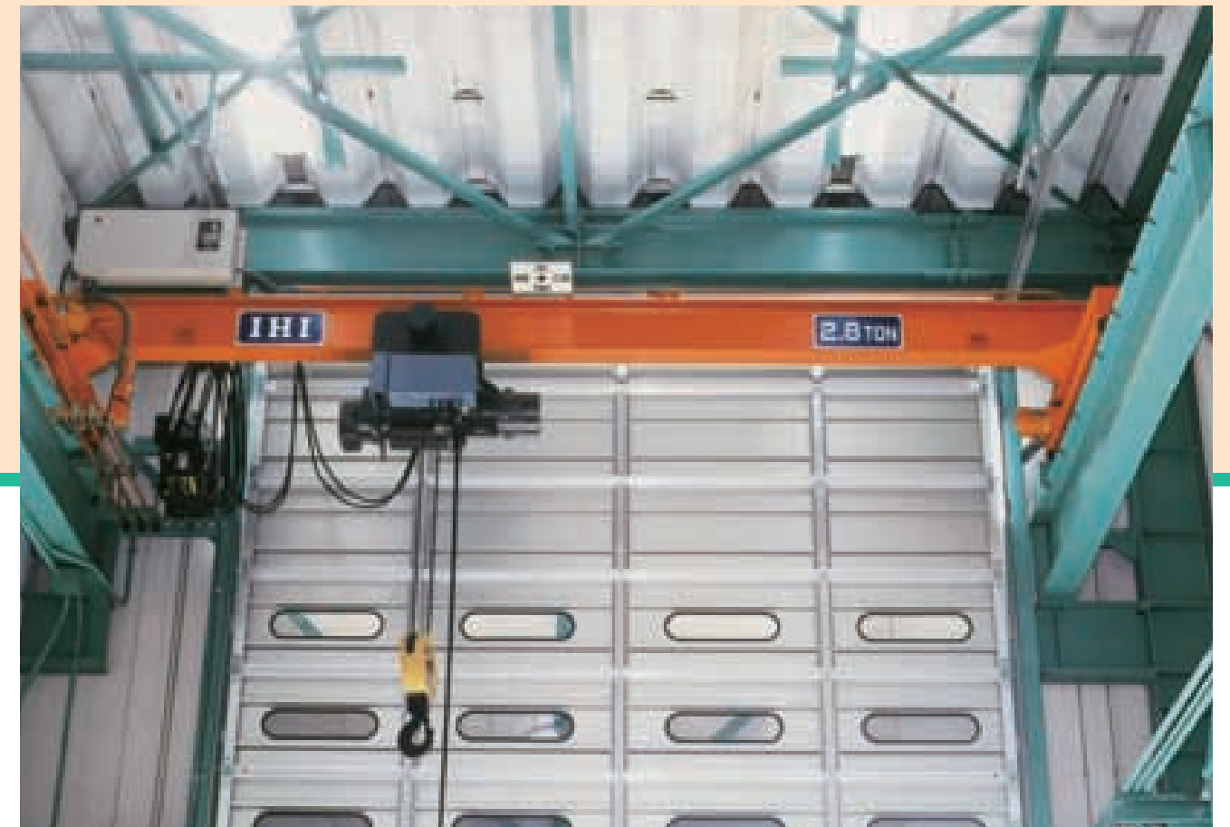
Overhead Traveling Crane with Mono Rail Hoist
